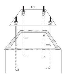
YOU ARE NOW FINISHED WITH THE INITIAL ASSEMBLY STEPS. DO NOT PRO-CEED WITH THE ASSEMBLY UNTIL THE CONCRETE HAS FULLY CURED. CUR-ING WILL TAKE A MINIMUM OF 72 HOURS. IN HUMID CLIMATES OR WET WEATHER, ALLOW ADDITIONAL TIME FOR THE CONCRETE TO CURE.
